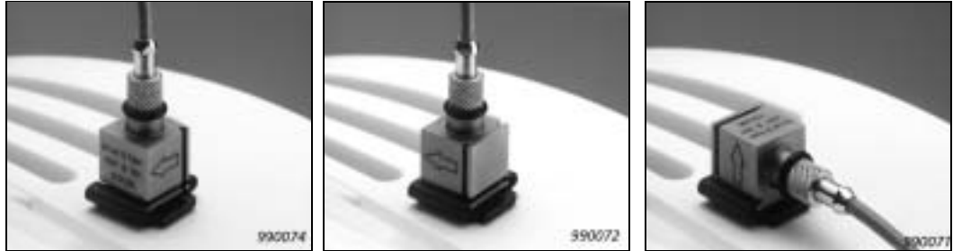
Fig. 14 Example of a triaxial measurement performed by rotating Type 4507B004 in the mounting clip
